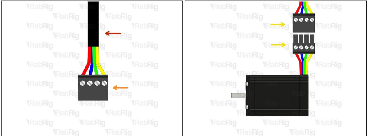
**i** Prepare the 4 wire cable for the Z stepper motor.
