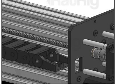
• Fit the Drop-in T-Nut mounted on the drag chain inside the 2040 slot and tighten the screw to lock it in place.
