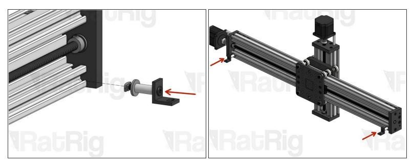
Attach the 2 Cable Tray Mounts at about 10mm from each end of the C-Beam. Tighten the screw while making sure the L bracket doesn't twist.
