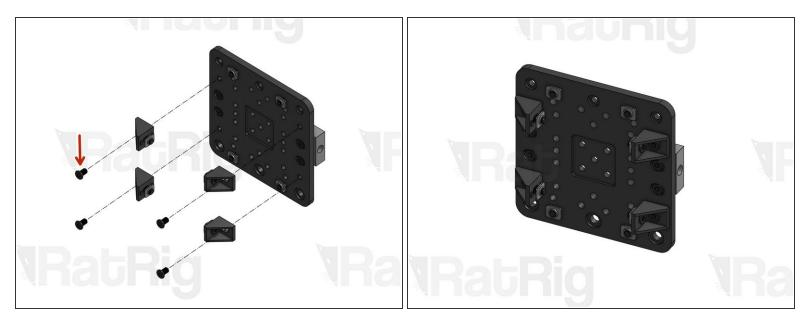
Low Profile Screw M5x8mm. Use them to attach the Cast Corners you set up on the previous step to the carriage.
