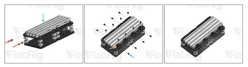
A Join the 2 X carriages together, noting the position of the Nut blocks in the picture.
