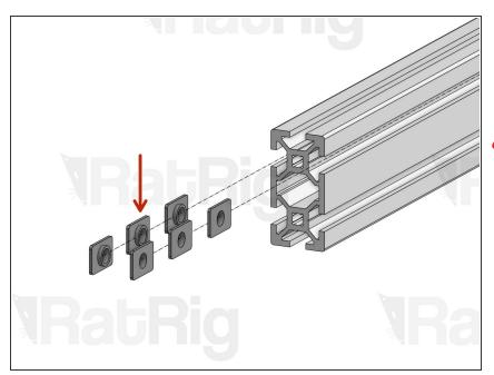
T-Nut M5. For the remaining 2 profiles, insert 3 T-Nuts on each side.
