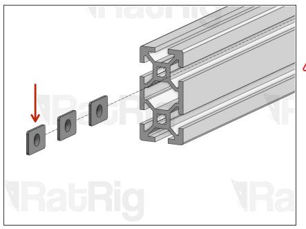
T-Nut M5. For 2 of the profiles, insert
