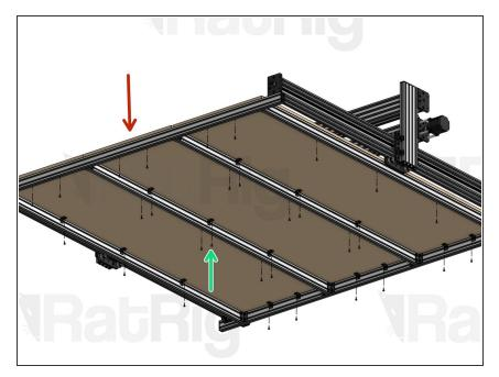
Round Head Cutting Screws. Use them to attach the board to the Single L Brackets.
