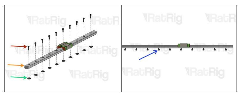
(i) Repeat this step for 3 Linear Rails (on a 300x300x300mm machine they will be 400mm long).
