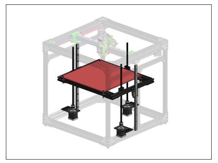
Remove all Z related parts from your current build, including the bed frame (items highlighted in the picture). You will reuse many of these parts in the new build, but in different places.
