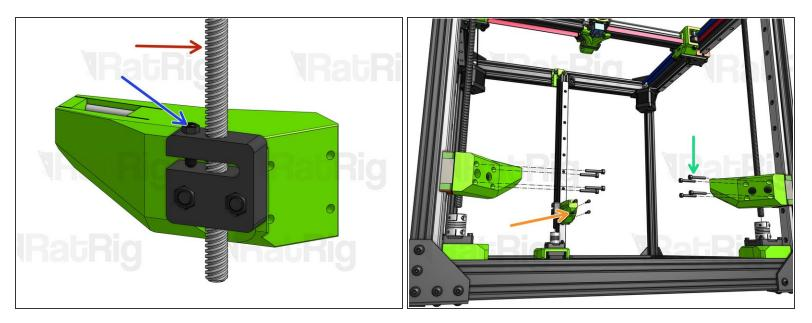
A CAUTION: if you have lead screws of different sizes, make sure you use the short one on the Back Z Arm. Note that this arm is different from the frontal ones.
