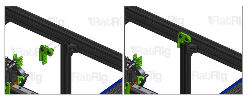
Fit the T-Nuts inside the slot and press the corner of the Back Cable Relief against the corner of the Back 2020 profile. Tighten the screws to secure in place.
