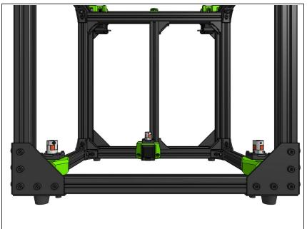
(i) In the final steps of the assembly the Z motor mounts will need to be adjusted in their XY positions to ensure the lead screws are parallel to the rails
