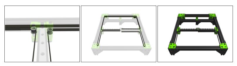
Fold the belts through the XY joiners so that all 4 ends end up in the middle of the X gantry.
