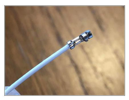
A perfect crimp. The first clamp holds the plastic, the second only wire. The round clutch is unharmed.
