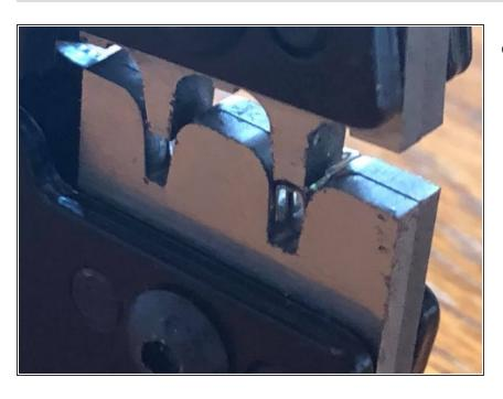
At first, press only two clicks so the pin is fixated in the wrench.
