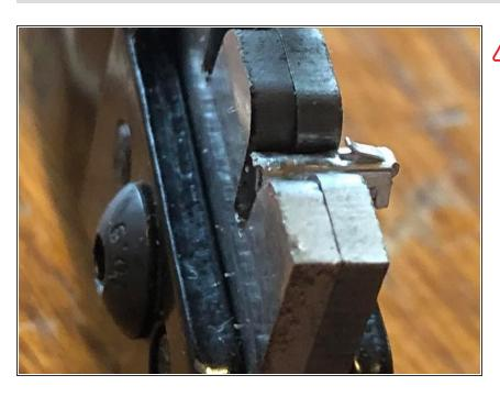
Match out: the bracket has a wide and a narrow half. Make sure the hook is unharmed.
