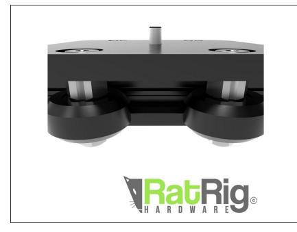
Before inserting your carriage on the main rail, use the 10mm wrench to turn each eccentric spacer to face outwards as shown. This means the stripe in facing away from the rail.
