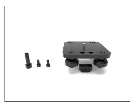
Grab the brake plate, 2x M4\*8mm cap head screws, and the big brake screw.
