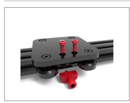
• Remove your slider's brake plate by unscrewing the 2 screws that hold it in place, using the **3mm Hex Key.**
