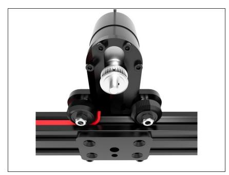
Slide the opposite tip of the Belt through the gap between the rail and the wheel of your slider's carriage.
