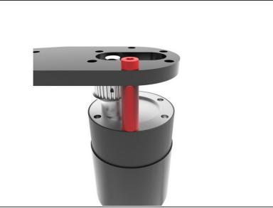
Pass one 25mm Screw through one of the holes on the Motor Plate, then through a black spacer and finally screw it into the motor. Repeat until you've used the four 25mm Screws and respective Black Spacers. Make sure you use the same holes from which you removed the original screws, on step 2.
